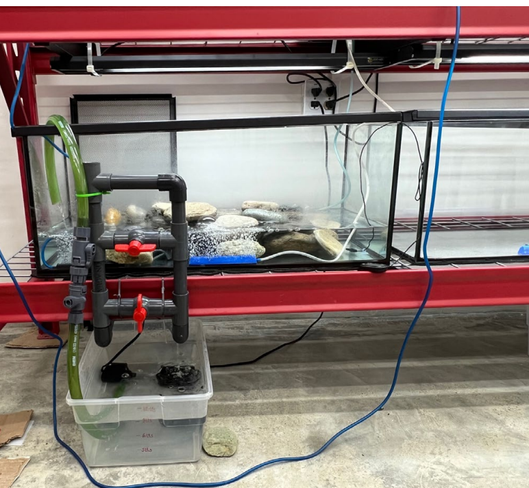
Tank for the reproduction of harlequin toads with water level control. Design adapted from the Panama Amphibian Rescue Center. Photo: Margarita Lampo.
