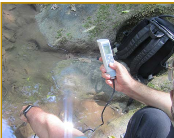
Testing water quality (pH, salinity, oxygen, total dissolved solids [TDS], temperature, and conductivity) inside water pool. Photo: Haji Gholi Kami
