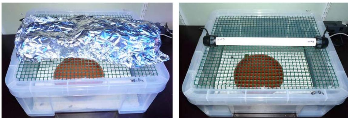
*Above: A highly adaptable and robust habitat for testing UV-B is a plastic box with a hole cut in the lid and plastic garden mesh covering. A fluorescent light can be placed over the top of the mesh and then covered with an aluminium foil cover. The aluminium cover reduces dispersion of the light and increase UV-V in the box by 40%.*
