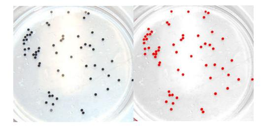
ImageJ<sup>™</sup> program allows for easy counting of eggs. It automatically counts all objects it recognizes in the final red image (right).
