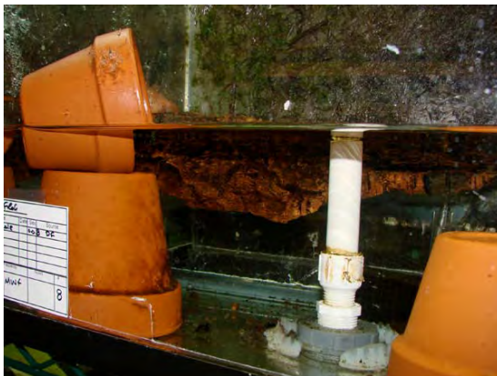
Figure 6. An internal standpipe used to regulate the water level inside a terrarium. (Photo: R. Gagliardo)
