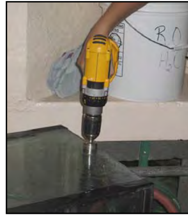
Figure 5. Demonstration of how to drill a hole in a glass aquarium using a diamond-tipped drill bit. Photographed at the AZA Amphibian Biology, Conservation, and Management course where everyone gets to try their hand at drilling a tank. (Photo: J. Pramuk)
