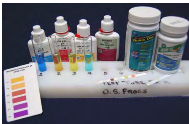
Figure 14. Two types of colorimetric water quality testing kits: on the left are freshwater liquid tests that are mixed in a test tube; on the right are two types of paper strip testing kits (5-in-one and chlorine/chloramine). Both tests result in a colored sample that is compared with a chart to reveal the level of pH, or parts per million (ppm) of the chemical being tested. These tests are relatively inexpensive and an easy way to perform quick tests of water quality which are invaluable for troubleshooting and
